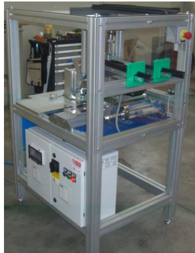
Machine with cutting heads for steel-reinforced rubber profiles
