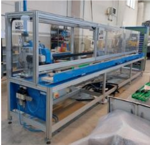
Die-cutting machine for rubber profiles with steel core
