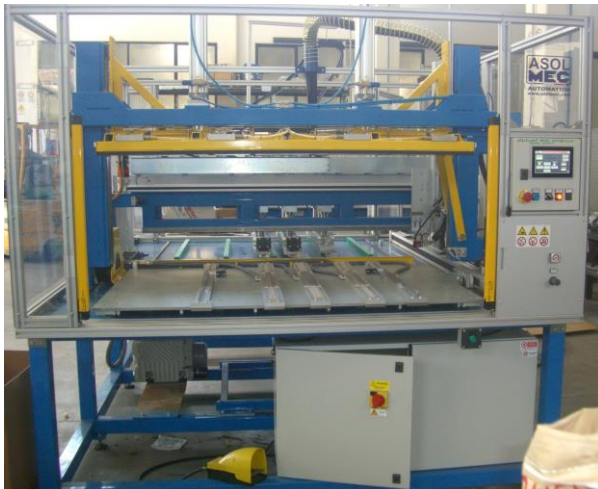
Machine for cardboard spine creasing, glue application, and mechanical cardboard-to-sheet bonding
