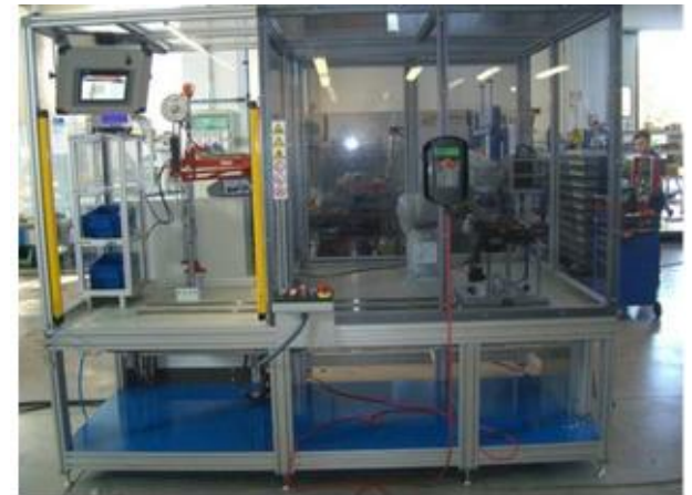
Robotic station for automotive air filter assembly, marking, and quality control
