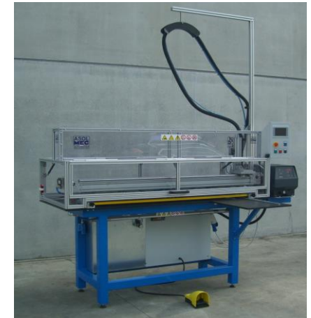
Folder flap folding machine following adhesive application
