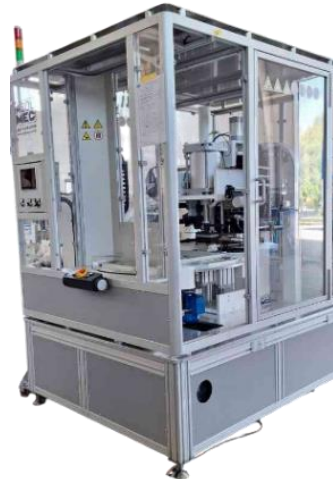
Automated transfer machine for hot stamping application, equipped with a rotary table.
